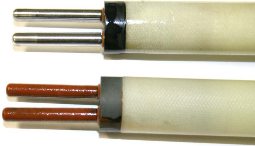
Figure 6: Comparison of corrosion on LPR probes in VpCI and nitrogen blanket protection system, showing no rust formation on VpCI protected steel samples, while nitrogen blanket protected steel samples covered with a thick red rust.
